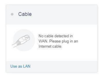
Plug the Ethernet cable into the WAN port of the router. The information of your connection will be shown on the Cable section. DHCP is the default protocol.
